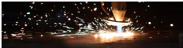
GAS/OXY-FUEL CUTTING Cost-effective method for cutting thick steel sections with excellent edge quality.
