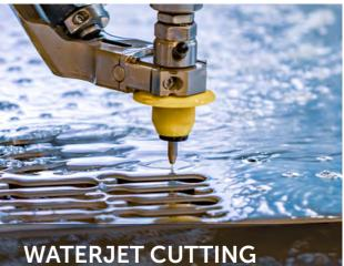
Cold-cutting technology for heat-sensitive materials, ensuring no distortion or hardening.
